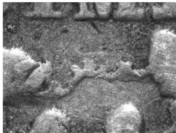
Die crack connecting left and right wreath leaves
